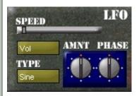
LFO controls the low frequency modulation which are used to change properties values overtime
